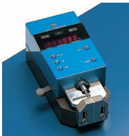
These highly accurate digital micrometers use UNION TOOL's own spindle structure (SF-class) crossed roller guides, together with precise glass scales. Use the lever to open the probes, then place the object to be measured between them, so that measurement is carried out under a constant pressure; the value is displayed digitally.
