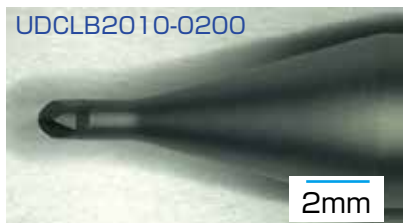
Tool #1 milled 3.5mm depth.
