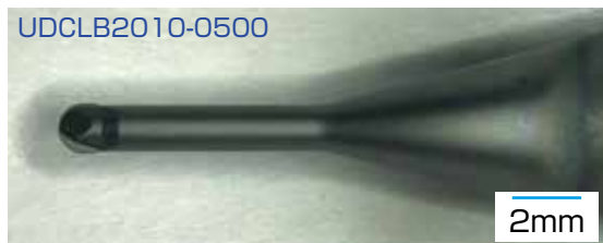
Tool #2 milled 131.9mm 3 in 76.5 minutes.
